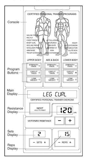
The heart of the resistance system is the digital resistance training console. The console offers both a manual mode and nine workout programs. When the manual mode is selected, the resistance setting can be changed with the touch of a button. When a program is selected, the console will guide you through an effective upper body, ab and back, or lower body workout.
